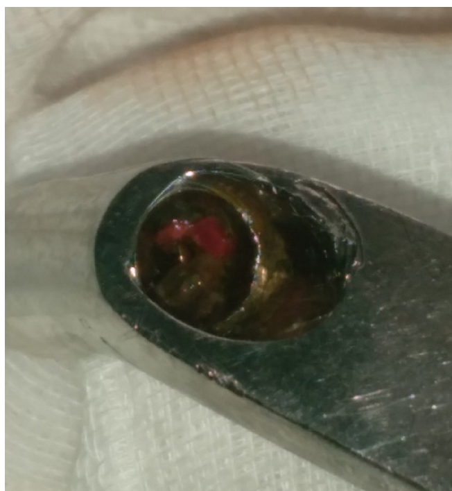
Figure 2. Photograph showing cold welding of barrel plate to Richard screw seen end on
